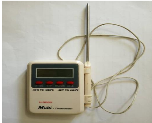
Figure 1: Digital thermometer with probe and sensor brand H-926.
